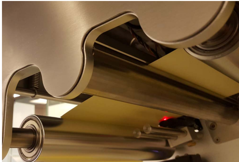
Media going through between the NIP clamps:
