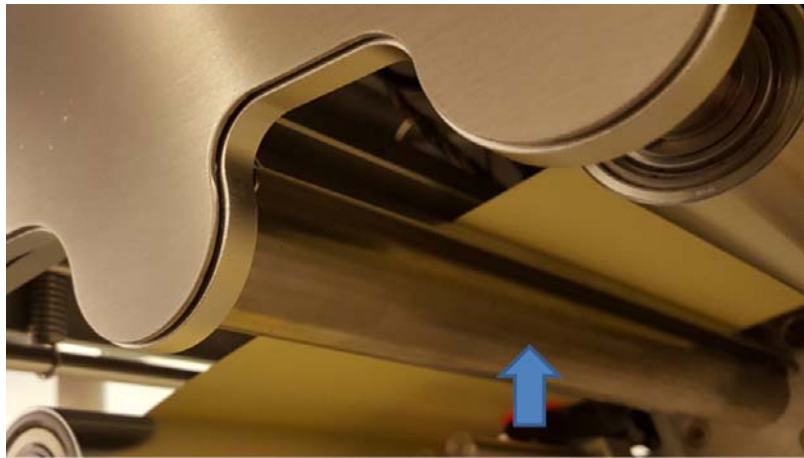
NIP metal roller marked with an arrow.
