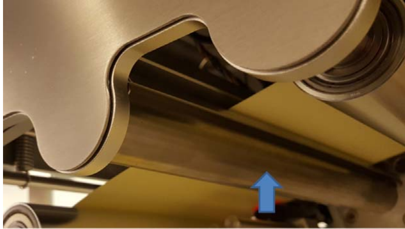
NIP clamp rubber roller marked with an arrow.
