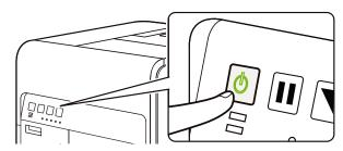
Cleaning is performed and the printer becomes ready for printing. When the printer is in the Online mode, the STATUS LED stays lit.
