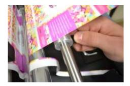
Once achived the desired cutting quality, fon both sides move the edges guides 5mm outside from the media edges.
