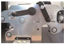
To properly load media, ensure that the nip roller and slitter module levers are in the open position.
