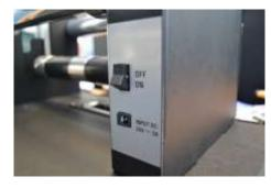
Connect included power supply to the unit and turn on through the main On/Off Switch.
